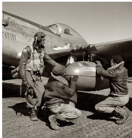
March 1945, Ramitelli, Italy. 332nd Army AF Fighter Group. "Tuskegee airman Edward C. Gleed of Lawrence, Kansas, Class 42-K, two crewmen adjusting an external 75 gallon drop tank on the wing of the P-51D Creamer's Dream."
